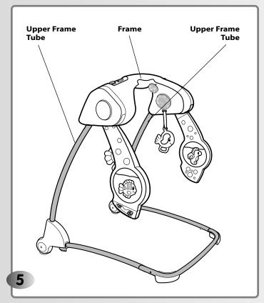
• Check to be sure the upper frame tubes are secure in the frame. If you can remove the upper frame tubes from the frame, you have not properly inserted the tubes into the frame. Remove the upper frame tubes from the frame and repeat Assembly step 4.
